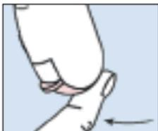
Gently close the battery compartment by pressing the bottom of the door upward with your finger tip. Do not force the door shut. If it does not close easily, check to see if the battery was inserted properly. When the battery door is completely closed, your hearing instrument is ready for use.
