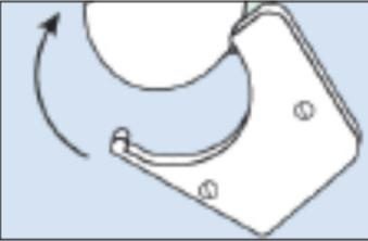
Take the audio shoe and hook the two nibs into the two small recesses of the hearing system housing. Slide the audio shoe towards the inner side of the hearing system housing until it snaps into the end position.
